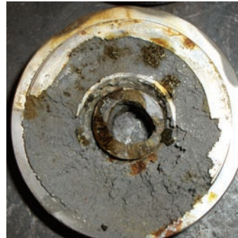
Fig 12 and 13 Original trim with severe cavitation damage
