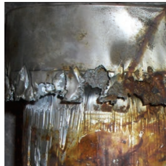
Fig 12 and 13 Original trim with severe cavitation damage
