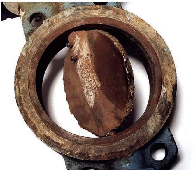
Fig 17 Cavitation damage to Butterfly valve
