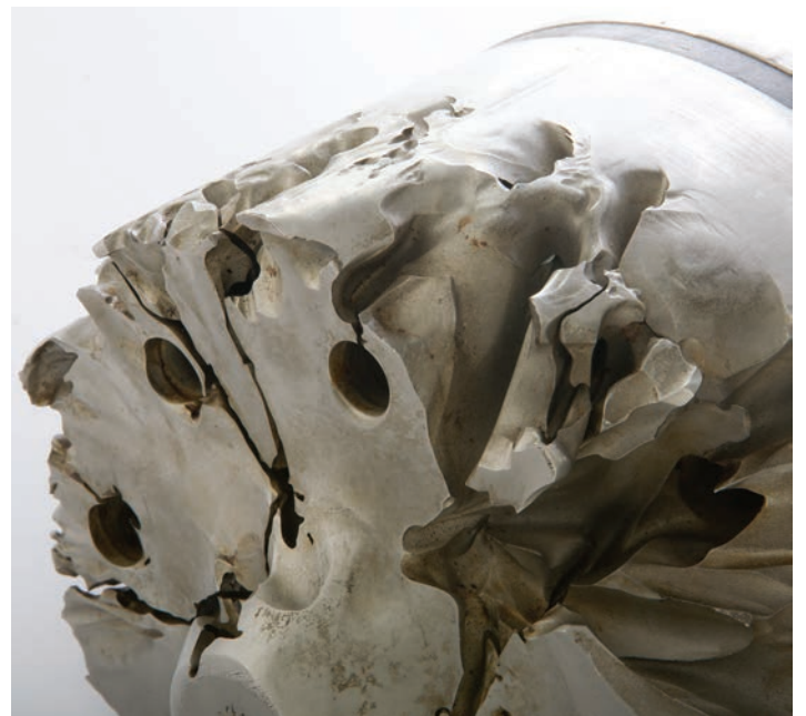
Fig 25 Fully stellited cage guided trim after two weeks operation
