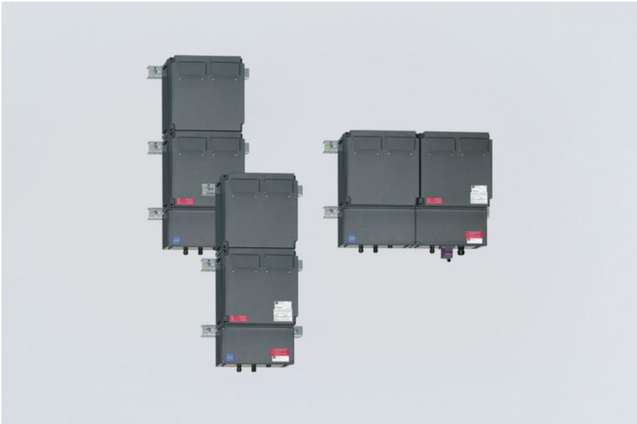
The R. STAHL Series 8316 battery box also provides a reliable back-up power supply in hazardous areas in continuous operation. It can be handled cleanly and safely since the gases generated during charging are recombined to form water in the closed battery system. Thanks to low self-discharge and protection against total discharge features, the battery has a stable cycle, is maintenance-free and has a long service life.
