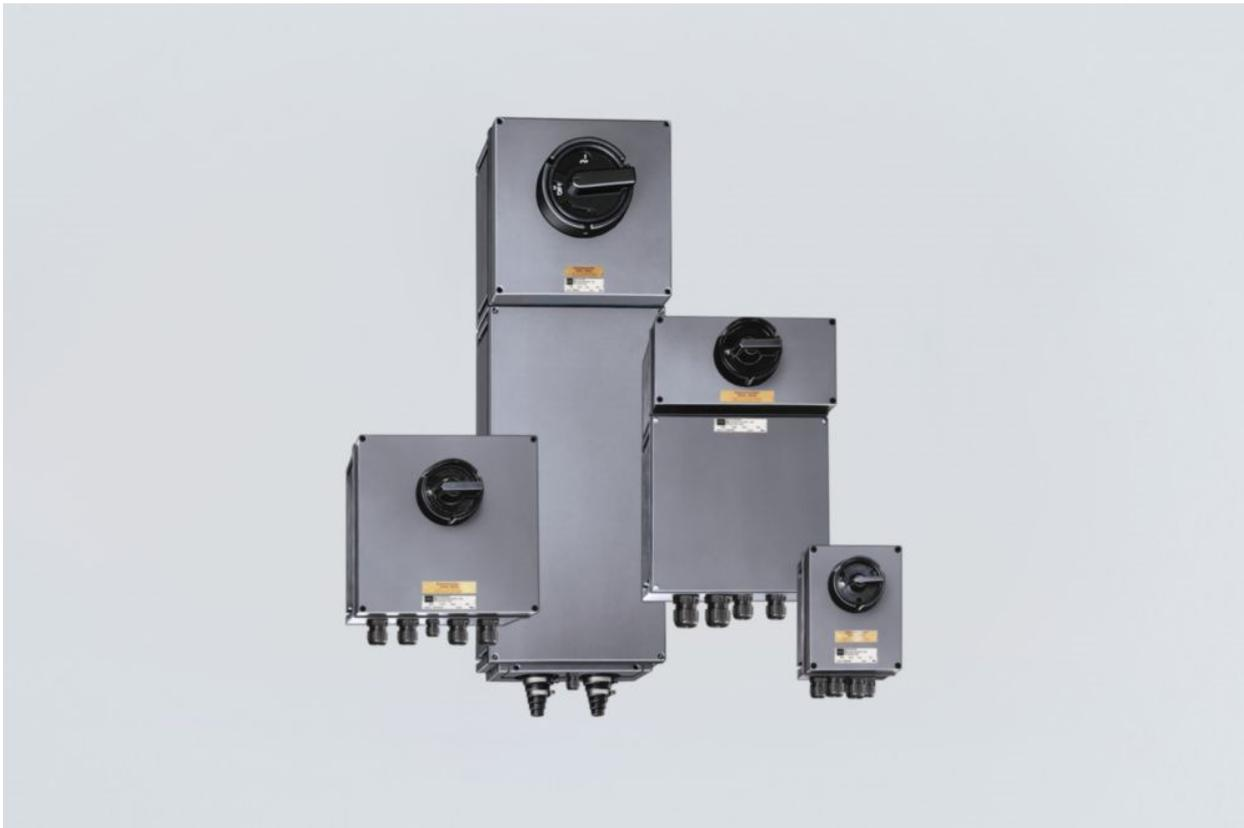
R. STAHL's robust load and motor switches can be used as mains connection switches for power distribution systems and motor circuits in hazardous areas. They have a switching capacity of AC-3 or AC-23 for switching motors. The standard variants are designed for rated operational currents of up to 80 A; versions with rated operational currents of up to 630 A are available on request.
