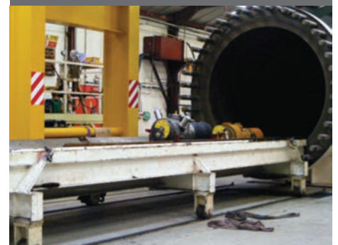
SUBSEA CHOKES ON HYPERBARIC CHAMBER LOADING BED
