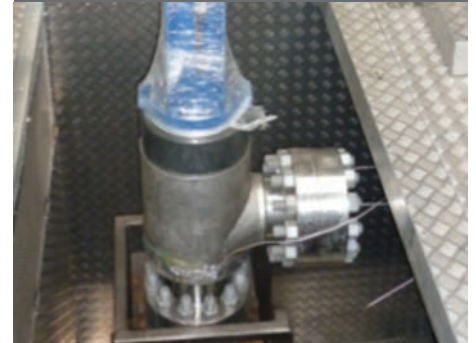
CHOKES IN ENVIRONMENTAL CHAMBER DURING PR2 QUALIFICATION
