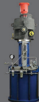
INTROSTEP SUBSEA ACTUATOR ON DOUBLE ACTING PISTON LOAD RIG
