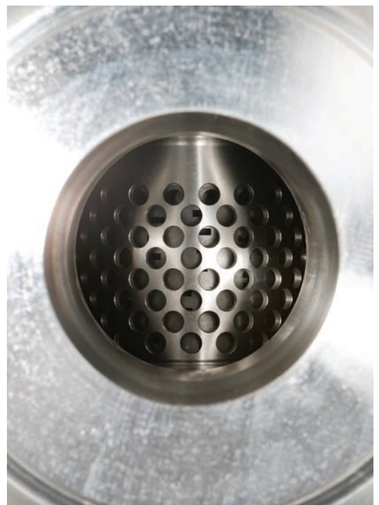
NON-COLLAPSIBLE TRIM DESIGN C/W METALLIC "BRICK-STOPPER"
