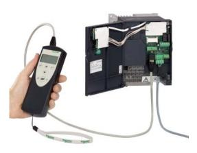
The dual port enables a dialogue tool and a communication network to be connected at the same time.
