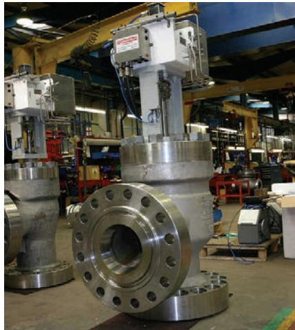
12" ANSI 1500 choke C/W electro-hydraulic actuator
