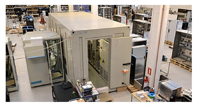
To reduce start up and commissioning on site we offer various integrated container/E-house solutions – what we call a "Plug and Play Solution" on site. The containers can be equipped with; Distribution panels, control panels, UPS system, air conditions etc.
