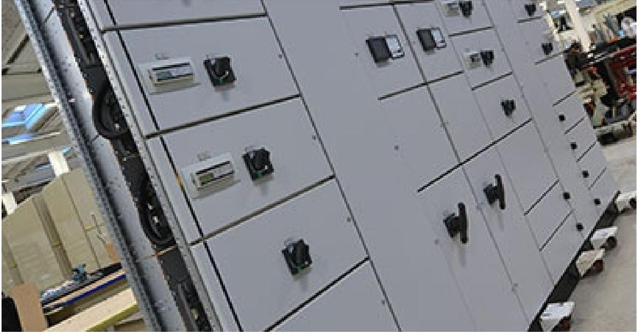
Complete unit substations can be constructed from the standard modular system.
