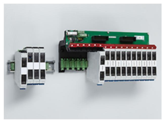
These isolators provide galvanic separation when they integrate field devices in process systems into automation systems. R. STAHL's ISpac isolator range is easy to use and boasts an impressive range of functions and a long service life.
