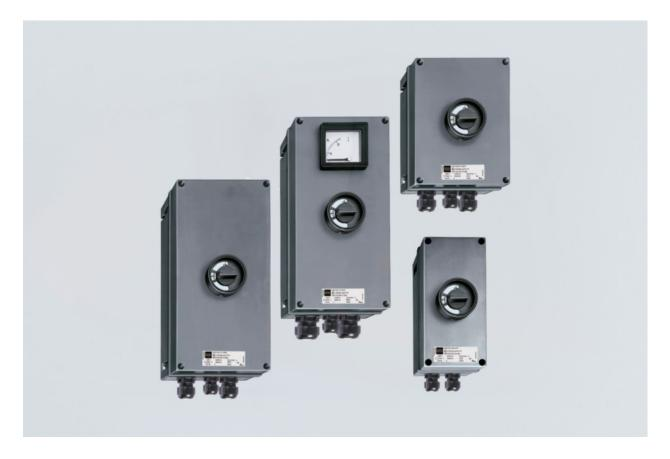
R. STAHL's moulded case motor protection circuit breakers offer reliable protection for Ex e and Ex d motors against short-circuiting and overloading in hazardous areas. They are available with a choice of different release types and, optionally, with an ammeter or auxiliary contacts. And thanks to their robust, polyester resin enclosure, they can be used in Zones 1, 2, 21 and 22.
